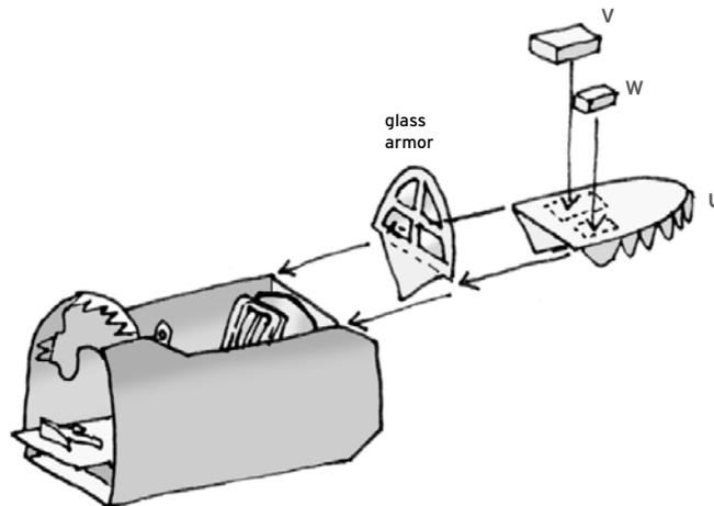
11. Glue the cockpit into the fuselage
