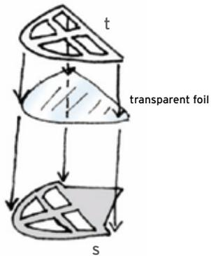
9. Main assembly. Glue the frames on the cockpit floor then add all else on top.
