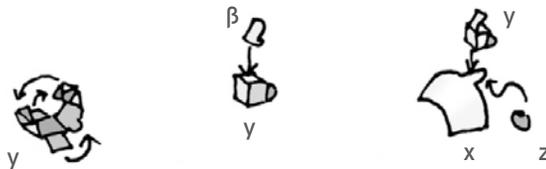
Glue the box, glue on the sight, glue both to the armature, then add the pillow from below
