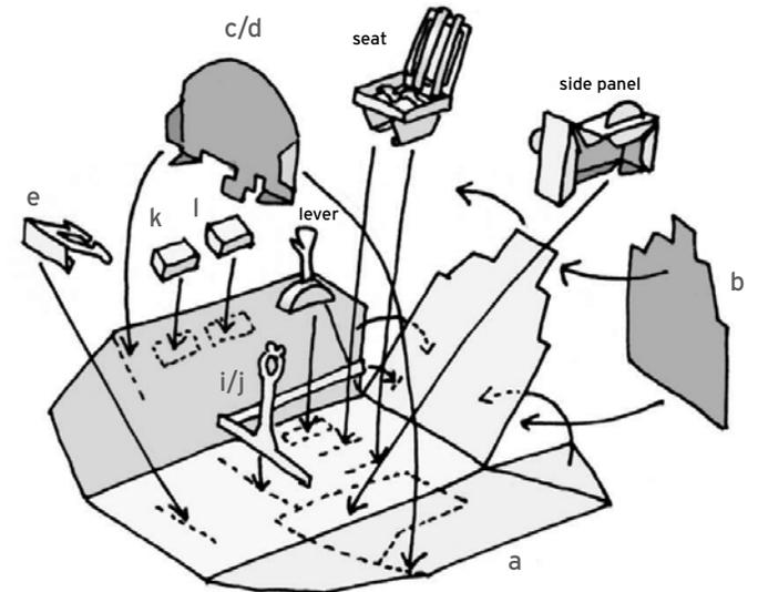
8. install the cockpit into the fuselage
